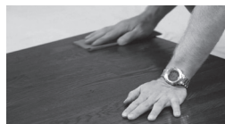
SAND ENTIRE SURFACE
